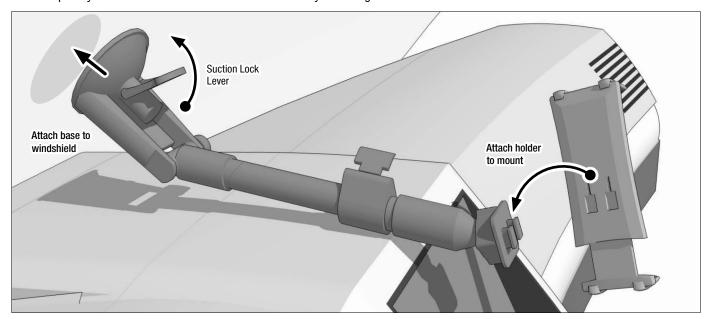
Adjust length of mount as necessary by unlocking extension arm. Lock arm when desired length reached. Insert device by pushing down on lower legs of spring-loaded holder.
